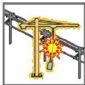
Hoist rope accesses dangerous area of high voltage power line with disastrous results
