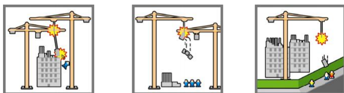
Hoist rope of high crane, hit by jib of low crane – the load is jolted and the banksman thrown off balance
